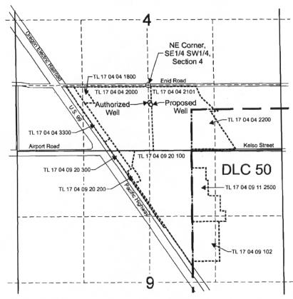
Authorized Well 6 is located 350 feet south and 30 feet east from the NE corner, SE1/4 SW1/4, Section 4.
