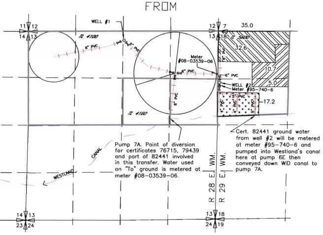
WELL #1 Located 270' South & 2540' West from the NË corner section 13, T3N, R28E, WM WELL #2 Located 1450' South & 3160' West from the N 1/4 corner section 18, T3N, R29E, WM
