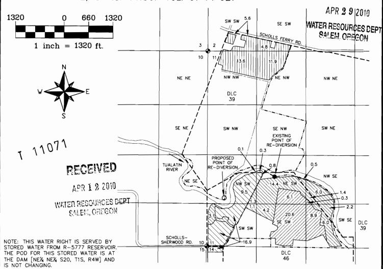
O POINT OF RE-DIVERSION WILL BE LOCATED 1300' NORTH AND 465' EAST OF THE SW COR. OF SECTION 11.
