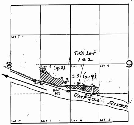
ZZ EXISTING TO REMAIN UNDER OLD DIV. PT. TRANSFER TO THE NEW DIV. PT. PT OF DIV TO REMAIN 750' S AND 1620' WEST FROM W1/4 CORNER SE 9 PT OF DIV TO REMAIN 1380' SOUTH AND 1020' EAST FROM W1/4 CORNER SEC 9 NEW PT OF DIV S008' 25"E 1096.98' FROM
