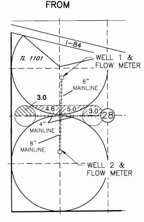
AUTHORIZED P.O.A. WELL 1 LOCATED 3700' N AND 1390' E FROM THE SW COR SEC 28 WELL 2 LOCATED 1650' N AND 1320' E FROM THE SW COR SEC 28
