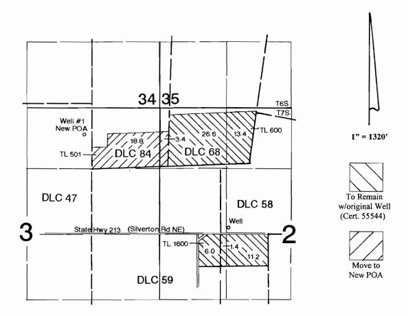
Exist'g Well is located in the 140' N & 1260' W from the center of Section 2. (SE1/4 NW1/4, Sec.2) Well #1 (New POA) is located 540' S & 1500' W from the NE corner of Section 3. (NW1/4 NE1/4, Sec.3)
