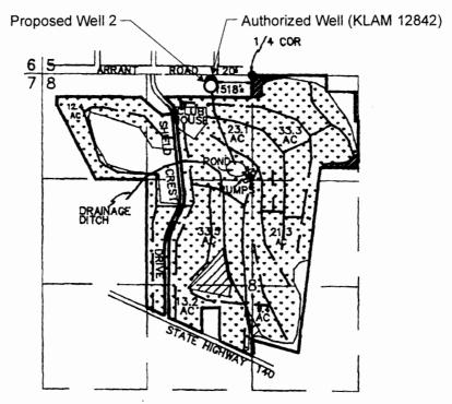
Authorized Well (KLAM 12482) is located 20 feet south and 518 feet west from the N 1/4 corner, Section 8. Proposed Well 2 is located 65 feet south and 519 feet west from the N 1/4 corner Section 8.
