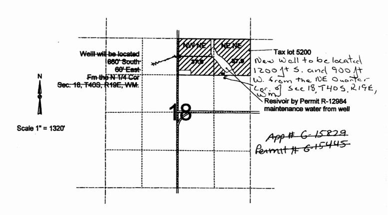
Water will be transported from well to reservoir by 6" pipeline
