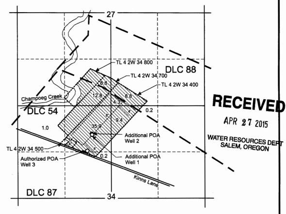
Authorized Point of Appropriation (POA), Well 3 is located 1,290 feet south and 680 feet west from the N 1/4 corner, Section 34.
