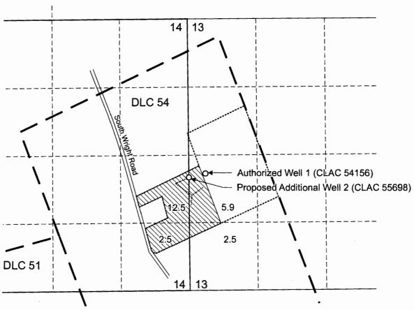
Authorized Well 1 (CLAC 54156) is located 2,360 feet north and 390 feet east from SE corner, Section 14. Proposed Additional Well 2 (CLAC 55698) is located 2,230 feet north from SE corner, Section 14.
