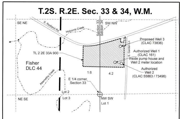
Authorized Well 1 (CLAC 161) is located 557 feet north and 250 feet east from the E 1/4 corner, Section 33. Authorized Well 2 (CLAC 55863 / 73496) is located 516 feet north and 345 feet east from the E 1/4 corner, Section 33.
