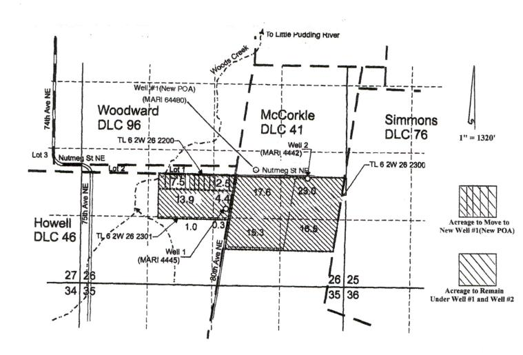
Well #1 (MARI 4445) is located 1520' N & 2365' W from the SE corner of Section 26. Well #2 (MARI 4442) is located 2130' N & 750' W from the SE corner of Section 26. Well #1 (New POA-MARI 64480) is located 100' N & 350' E from the NE corner of DLC 46.
