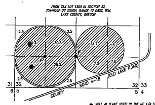
SW CORNER OF SECTION 32. ■ WELL #2 (LAKE 52371) IN THE SE 1/4 SW 1/4 SECTION 32, T27S R17E, W.M. LOCATED 1305 FEET NORTH AND 1320 FEET EAST FROM THE SW CORNER OF SECTION 32.
