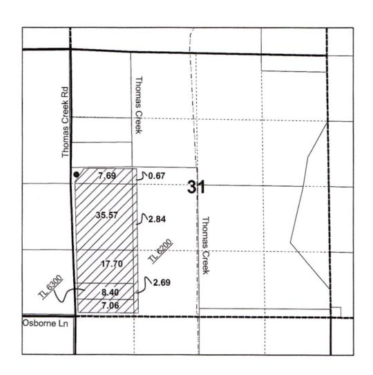
Proposed Well will be located in the SW1/4 of the NW1/4 of Section 31 T 38 S, R 20 E, WM 2532.5 ft South and 111.0 ft East Fm the Northwest Corner of Section 31
