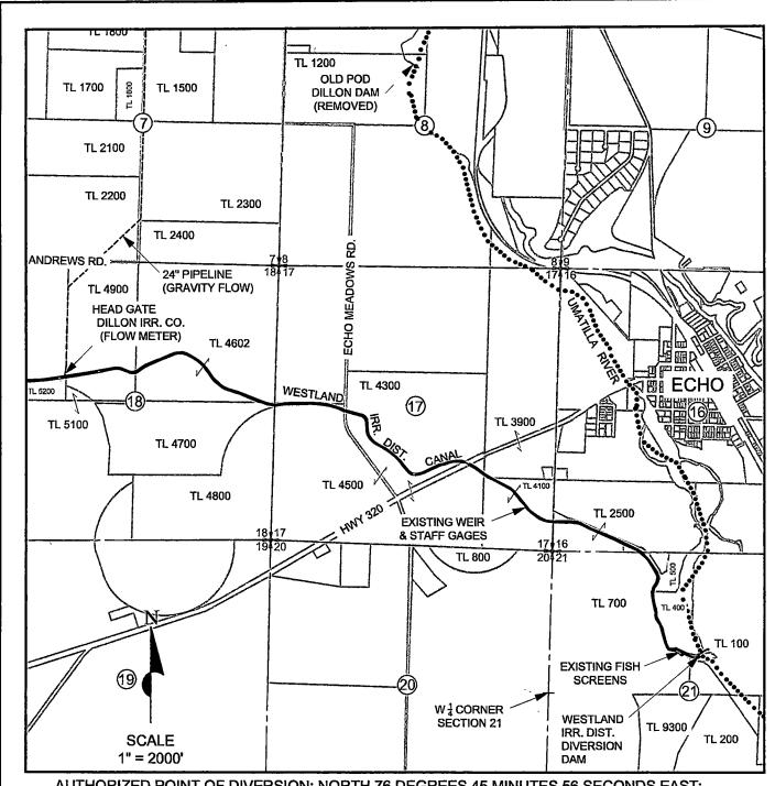
AUTHORIZED POINT OF DIVERSION: NORTH 76 DEGREES 45 MINUTES 56 SECONDS EAST; 2913.19 FEET FROM THE W 1/4 CORNER OF SECTION 21
