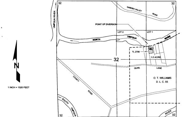
THE POINT OF DIVERSION IS LOCATED 600 FEET NORTH AND 1205 FEET WEST FROM THE EAST QUARTER CORNER OF SECTION 32; BEING WITHIN THE SE ¼ NE ¼, AS PROJECTED WITHIN O. T. WILLIAMS D. L. C. No. 55, SECTION 32, TOWNSHIP 26 SOUTH RANGE'6 WEST, W.M.; DOUGLAS COUNTY.
