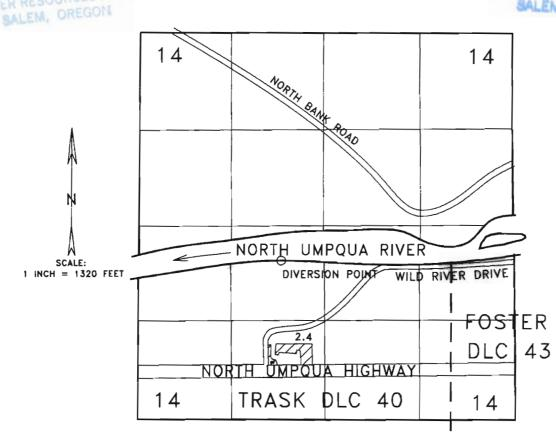
THE DIVERSION POINT IS LOCATED 2170 FEET NORTH AND 3160 FEET WEST FROM THE SOUTHEAST CORNER OF SECTION 14.
