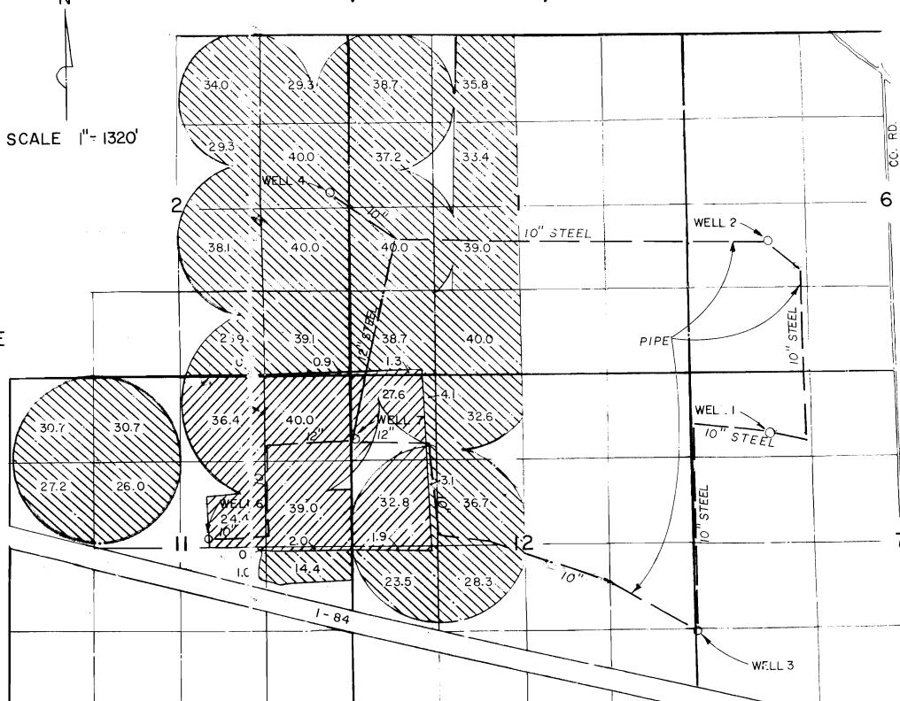
WELL 1 - 4340' N & 1830' W FROM S1/4 CORNER OF SECTION 7. WELL 2 - 2010' N & 1330' E FROM SW CORNER OF SECTION 6. WELL 3 - 1420' S & 40' E FROM W1/4 CORNER OF SECTION 7. WELL 4 - 180' N & 269' W FROM E1/4 CORNER OF SECTION 2.
