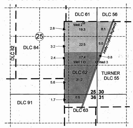
Well 1 is located 1,450 feet north and 580 feet west of the southeast corner of Section 25.
