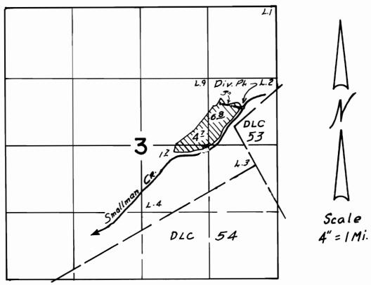
Div. Pt. loc. 430'N & 180'E FROMW'ly NW COR DLC 53
