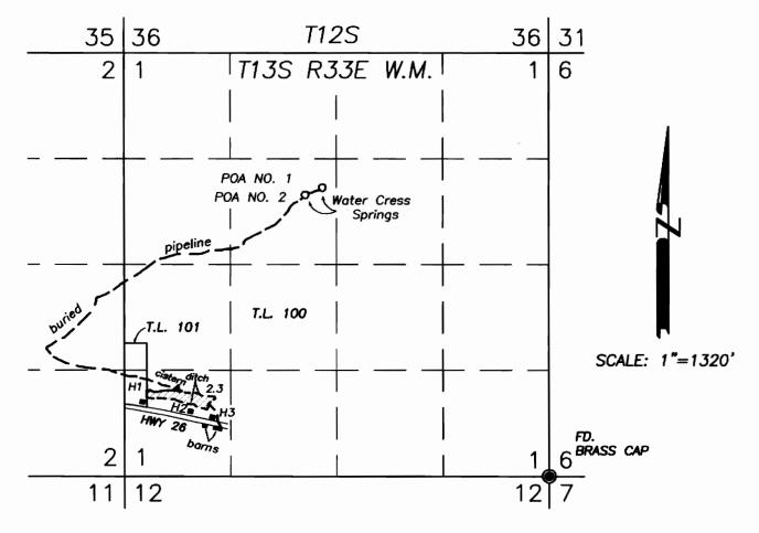
Point of Appropriation No. 1 is 3600' N. and 2830' W. of the SE Cor. Sec. 1. - T7420 Point of Appropriation No. 2 is 3510' N. and 3050' W. of the SE Cor. Sec. 1. - T7420
