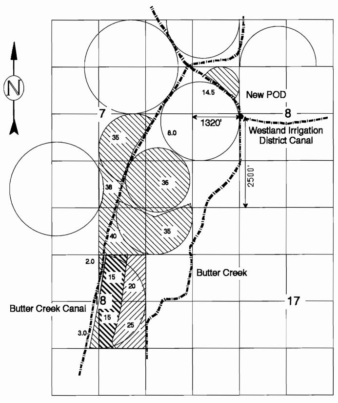
Point of Diversion Located 2500 Ft. North & 1320Ft. East of SW Corner of Section 8
