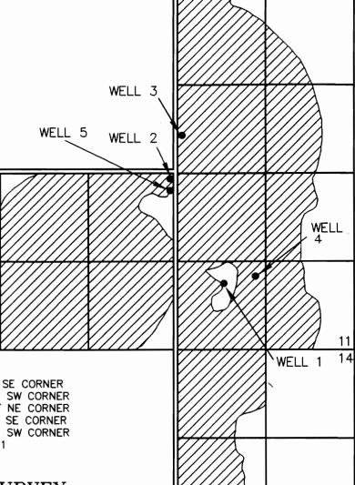
WELL 1, 980'N. & 1950'W OF SE CORNER WELL 2, 2550'N & 2550'E OF SW CORNER WELL 3, 2060'S & 2600'W OF NE CORNER WELL 4, 1090'N & 1480'W OF SE CORNER WELL 5, 2370'N & 2550'E OF SW CORNER ALL IN SECTION 11
