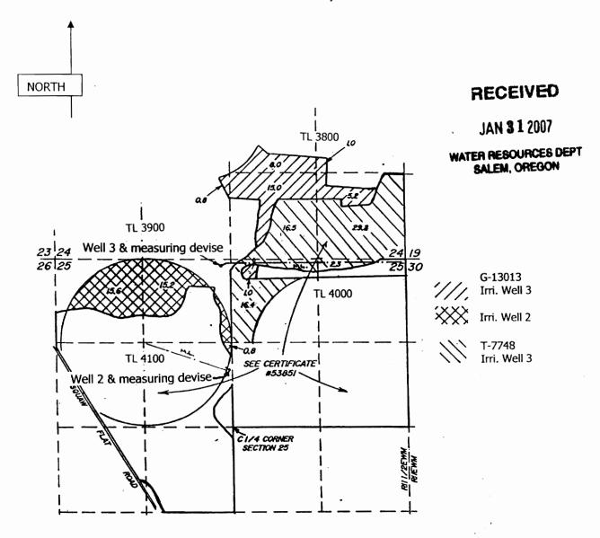
Well 2: 900' N & 50' W from the C  $\frac{1}{4}$  cor. Sec. 25 Well 3: 100' S & 2530' E from the NW cor. Sec. 25
