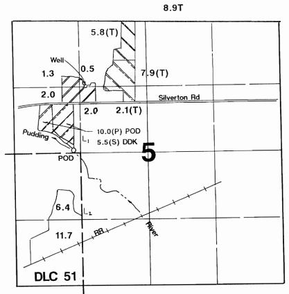
POD located 90'N & 4080'W from E¼ corner Section 5. Well located 1270'S & 1470'E from NW corner Section 5.
