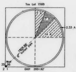
Point of beginning of survey is a 1/2" pin located at the SW Section Corner
