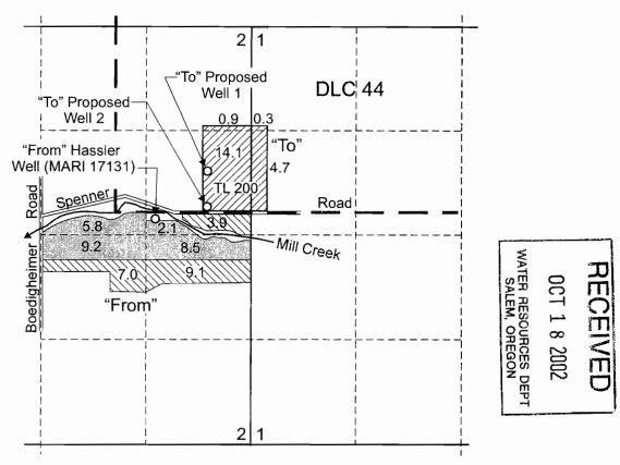
"From" Hassler Well (MARI 17131) is located 200 feet north and 1,430 feet east from the center of Section 2. "To" proposed Well 1 is located 800 feet north and 2,080 feet east from the center of Section 2. "To" proposed Well 2 is located 350 feet north and 2,080 feet east from the center of Section 2.
