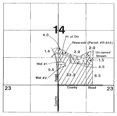
Well #1 located 1125'N & 80'E of \$1/4 corner Section 14. Well #2 located 925'N & 310'E of \$1/4 corner Section 14. POD located 1170'S & 180'E from center of Section 14.
