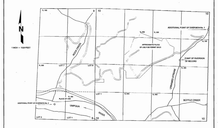
THE ORGINAL POINT OF DIVERSION ON THE UNNAMED STREAM IS LOCATED 2480 FEET SOUTH AND 3950 FEET EAST FROM THE NORTHWEST CORNER OF SECTION 10, WITHIN THE SE'A NE'A;
