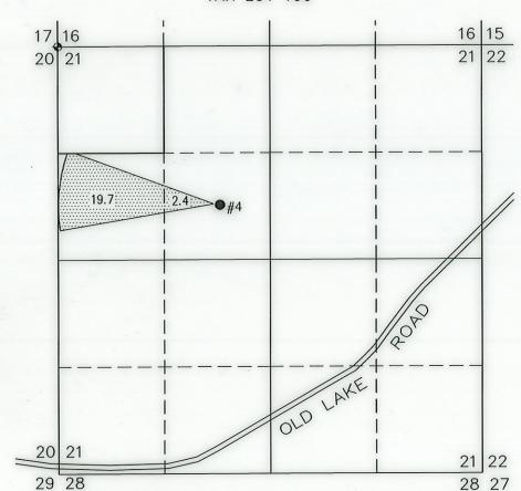
■ #4 (LAKE 1411-G8199) EXISTING WELL IN THE SE 1/4 NW 1/4 SECTION 21, T28S R16E, W.M. LOCATED 1990 FEET SOUTH AND 3280 FEET WEST FROM THE NE CORNER OF SECTION 21.
