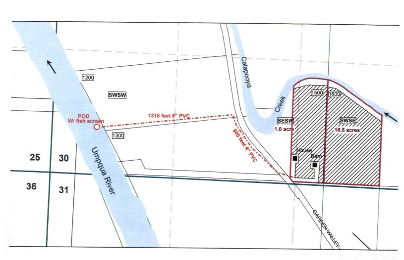
Point of Diversion is 462 ft North and 560 ft East From the SW Corner of Section 30
