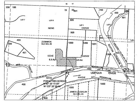
POD IS LOCATED 3000 FEET SOUTH & 80 FEET EAST OF NW CORNER OF SECTION 20 WITHIN DLC NO. 45.
