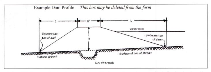
7. Provide a drawing showing the cross section of the dam at the maximum section indicating details and dimensions. The drawing should be drawn at a standard even scale.
