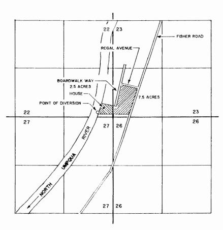
THE POINT OF DIVERSION IS TO BE LOCATED 110 FEET NORTH AND 420 FEET WEST FROM THE SOUTHEAST CORNER OF SECTION 22, BEING WITHIN THE SE 1/4 OF THE SE 1/4 OF SECTION 22, TOWNSHIP 26 SOUTH, RANGE 6 WEST,W.M.
