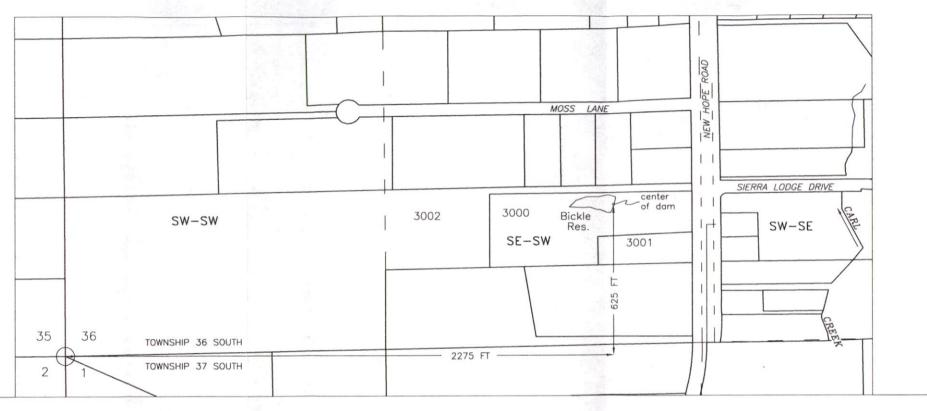
CENTER OF DAM - SE/SW, Section 36, T36S R6W, WM. 625 FEET NORTH & 2275 FEET EAST FROM THE SW CORNER OF SECTION 36
