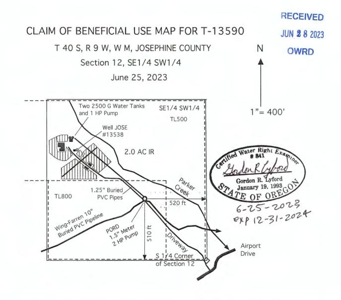
• Point of re-diversion from the 10" Wing-Farren pipeline, 2 HP pump, and 1.5" water meter. The PORD is 510 feet north and 520 west from the south 1/4 corner of Section 12.
