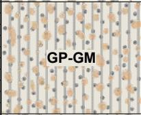
34.0 - 36.0 ft: Very loose, dry, light brown to gray, poorly graded GRAVEL with sand and silt (GP-GM), few silt, some sand is very fine to medium, subrounded to subangular, gravel is fine, subrounded to angular, trace cobbles (<4 in) [MISSOULA FLOOD DEPOSITS] | 50       | 40     | 10     |                               |  |
