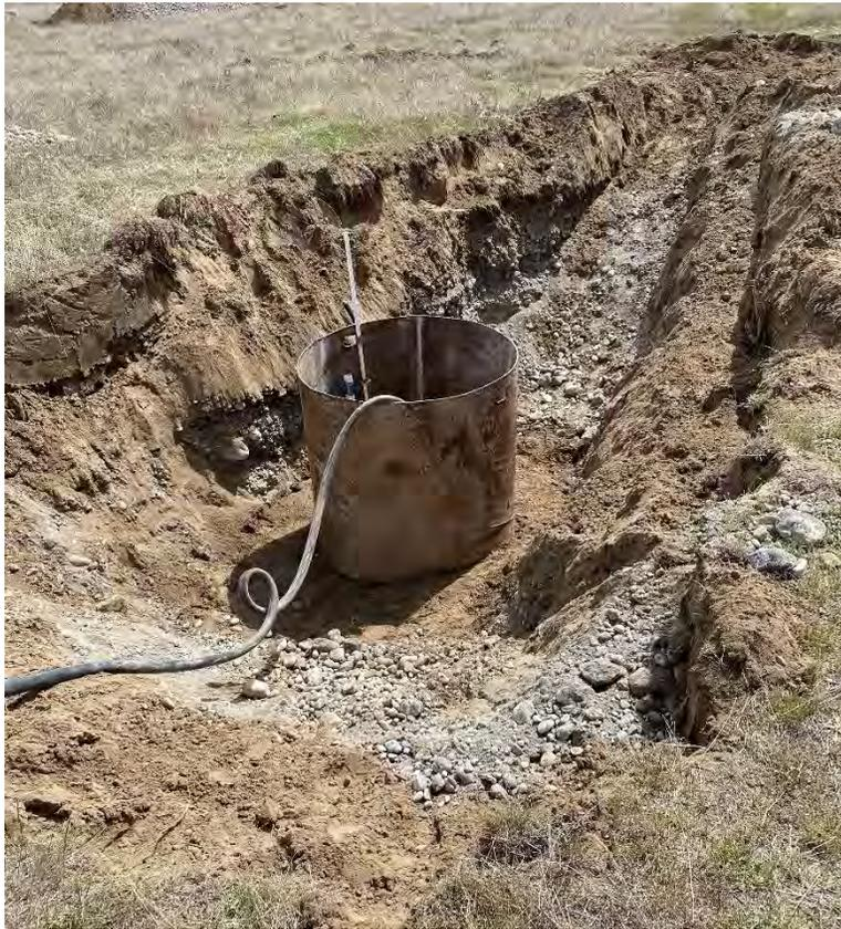
Figure 1. TP-16 infiltrometer test
