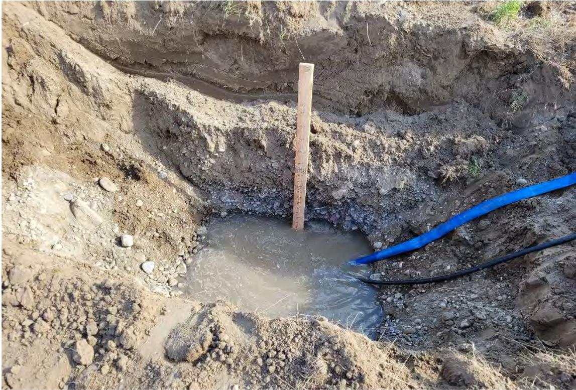
Figure 2. Example modified test pit infiltration measurement (TP-1 at 5.3 ft bgs)
