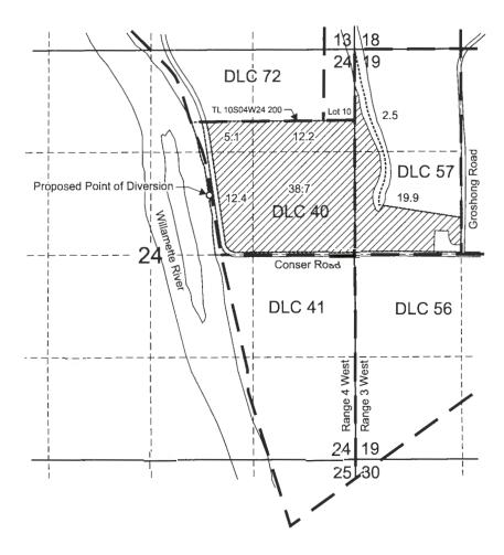
Proposed Point of Diversion is located 1,870 feet south and 1,880 feet west from the NE corner, Section 24.
