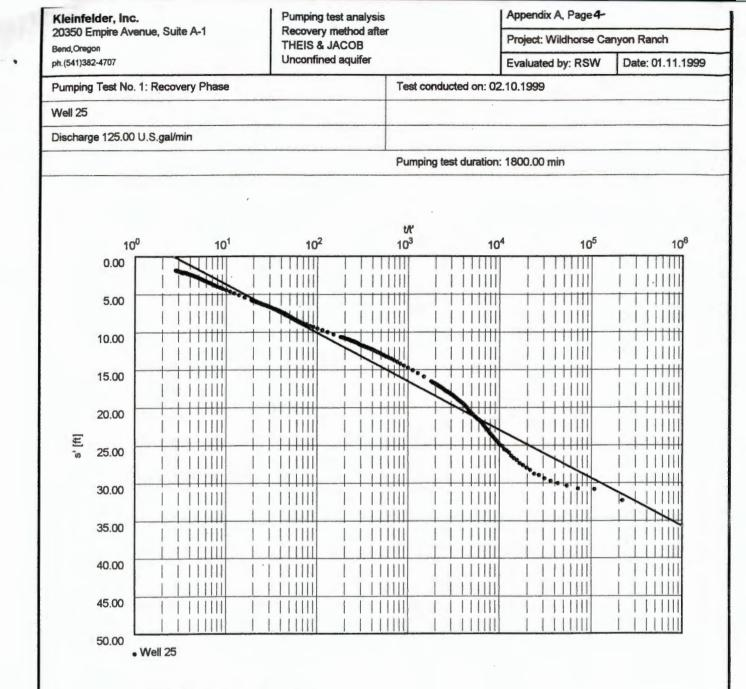
Transmissivity [ft²/min]: 4.76 x 10-1
