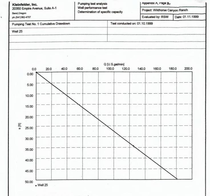
specific capacity C [ft²/min]: 4.85 x 10-1
