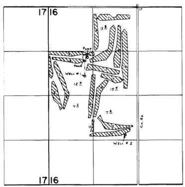
WELLS Loc: #1-2050'S. \$1560'W. #2-3780'S. \$360'W. ALL FROM N. 4 COR. SEC. 16. PUMP LOC: 1500'S. \$1480'W.
