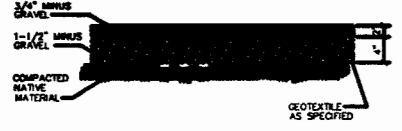
6. GRAVEL MAINTENANCE ROAD SECTION NTS
