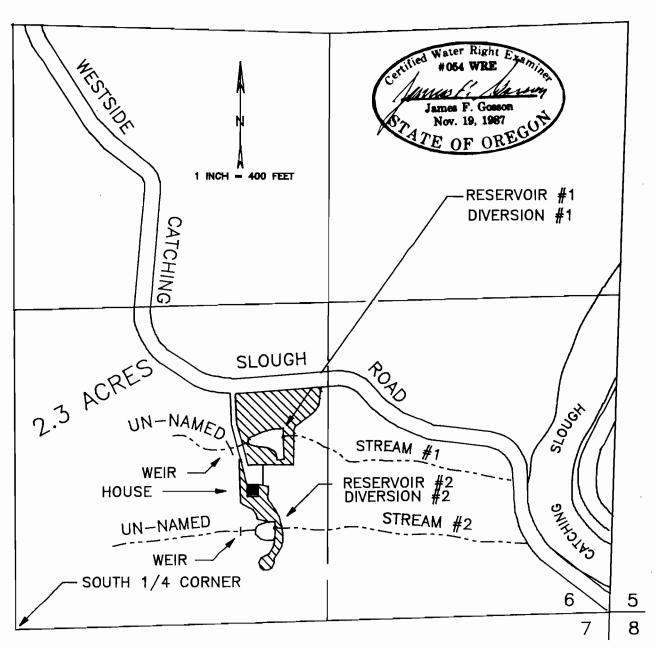
DIVERSION #1 IS LOCATED 740 FT. N & 1090 FT. E, DIVERSION #2 IS LOCATED 360 FT. N & 1060 FT. E, BOTH FROM THE S 1/4 COR. S6, BEING WITHIN SW1/4 SE1/4 S6, T26S, R12W, W.M., COOS COUNTY.
