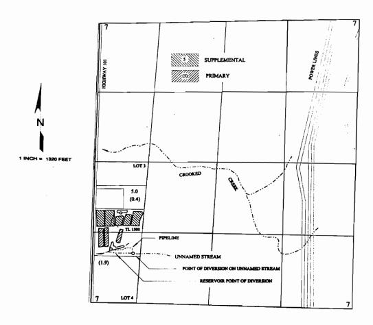
THE POINT OF DIVERSION IS LOCATED 1,000 FEET NORTH AND 840 FEET EAST AND BANDON RESERVOIR IS LOCATED 1,090 FEET NORTH AND 400 FEET EAST, BOTH FROM THE SOUTHWEST CORNER OF SECTION 7 AND WITHIN THE SW% SW% (LOT 4) OF SECITON 7, TOWNSHIP 29 SOUTH, RANGE 14 WEST, W.M.; COOS COUNTY.
