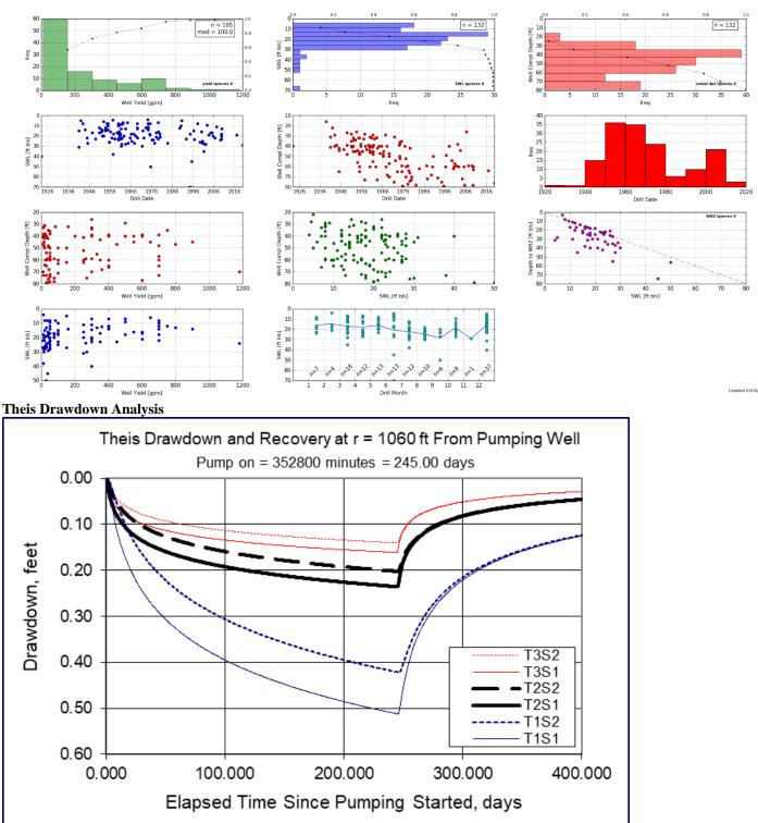
Radial distance from pumping well (r)=1,060 ft [estimated radial distance to nearest user, MARI 5330] **Pumping Rate (Q)= 0.272 cfs (~122 gpm) \***
