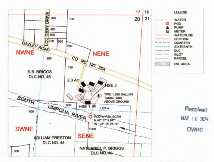
POD IS LOCATED 1408 FEET SOUTH & 723 FEET EAST OF NE CORNER OF SECTION 20 AS PROJECTED WITHIN GLOT 4.
