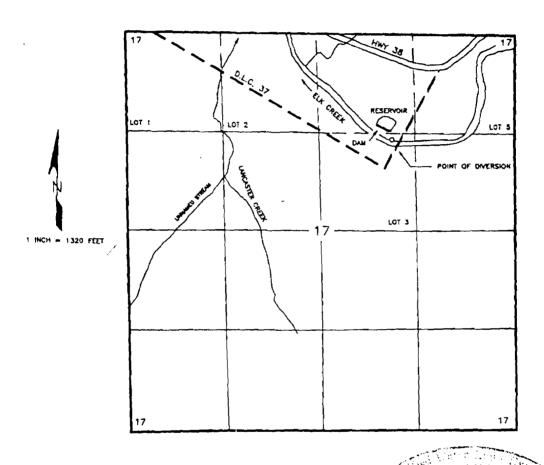
THE RESERVOIR IS TO BE LOCATED WITHIN THE NW% NEW OF SECTION 17, TOWNSHIP 22 SOUTH, RANGE 6 WEST, W.M.; THE CREEK POINT OF DIVERSION IS TO BE LOCATED 1450 FEET SOUTH AND 1680 FEET WEST FROM THE NORTHEAST CORNER OF SECTION 17, BEING WITHIN THE SW// NE// OF SECTION 17, TOWNSHIP 22 SOUTH RANGE 6 WEST, W.M., DOUGLAS COUNTY.
