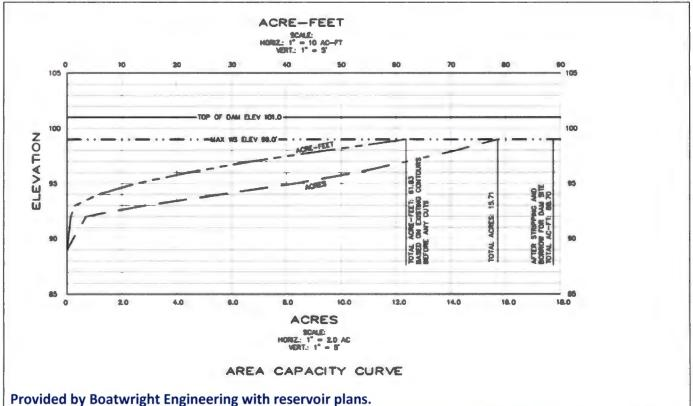
\*The area capacity curve shown above was developed prior to construction of the reservoir. After the reservoir was constructed, Boatwright Engineering determined that at full stage the constructed reservoir stores 90.0 acre-feet.
