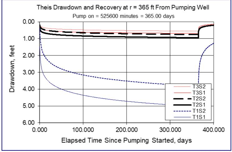
Radial distance from pumping well (r)=365 ft [estimated radial distance to nearest user, MARI 69448] **Pumping Rate (Q)= 0.038 cfs (~17 gpm) \***
