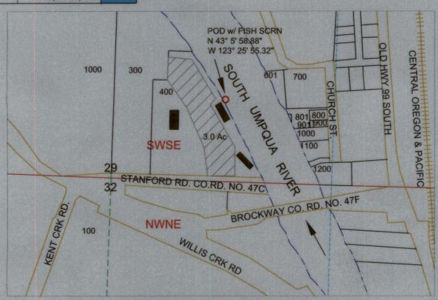
POD IS LOCATED 543 FEET NORTH & 642 FEET EAST OF S1/4 CORNER OF SECTION 29.
