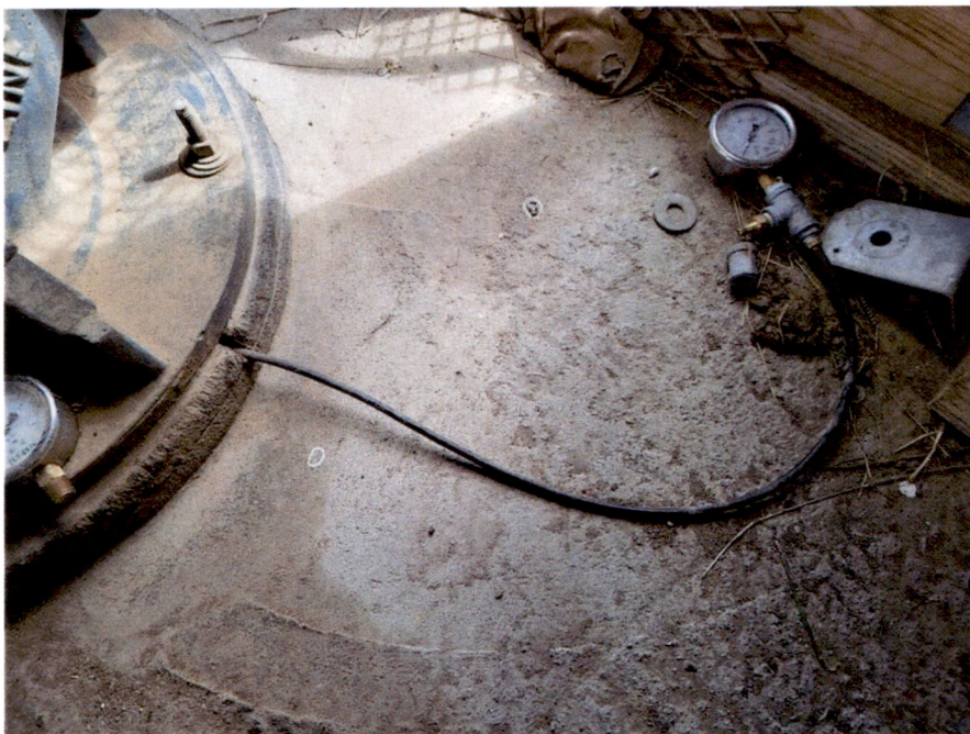
Pressure Gauge and Line for Water Level Measurement
